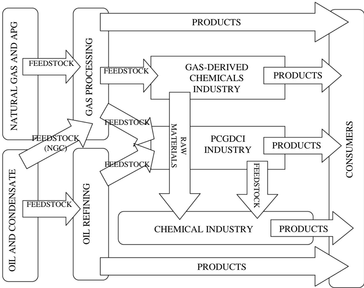
**Fig. 1 Emerging Structure of the CROGRPGDCI Sectors**
